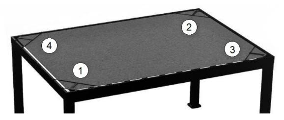
BUCKLE AND TIGHTEN THE STRAPS IN A CRISS-CROSS ORDER. SEE VIEW ABOVE. THIS WILL ENSURE THE SHADE IS EVENLY CENTERED ON THE PERGOLA.
